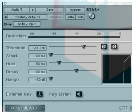
Figure 4-4: The gate plug-in lets you filter out noise below a certain level.
